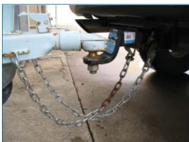
Figure 4. Safety chains in a crossing pattern
