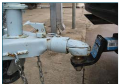
Figure 3. Collar moved into place to hold hitch
