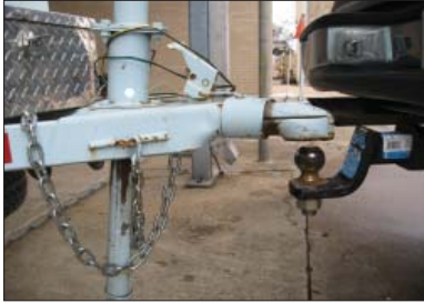
Figure 1. Align trailer hitch over ball on vehicle
