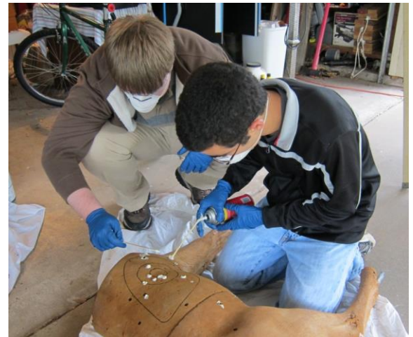
Figure 3 - Spray foam insulation was used to fill holes.
