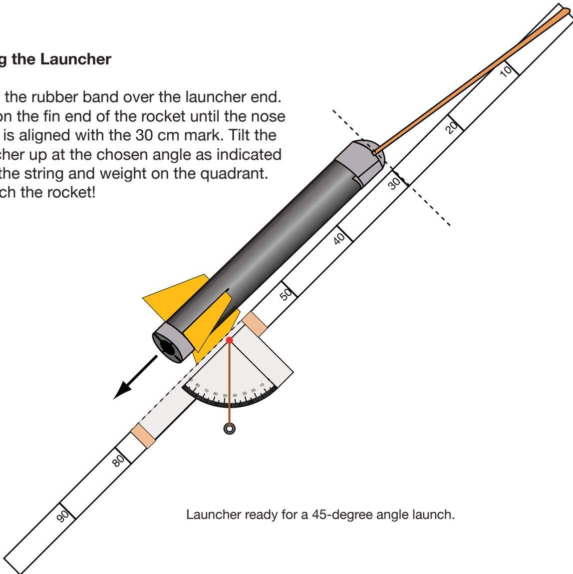
Launcher ready for a 45-degree angle launch.
